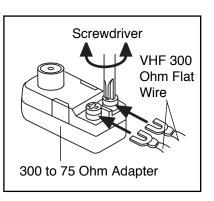
2. Connect the 300 to 75 ohm adapter to the 75 ohm antenna terminal on the treadmill. (See assembly drawing 6 on page 8 for the location of the terminal.)
